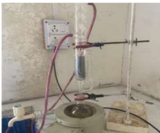
Fig.03: Extraction of Giloy by Soxhlet Apparatus
