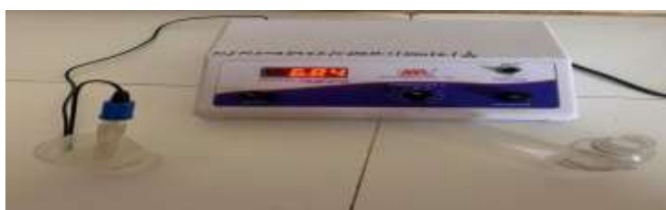
Fig.04: pH was measured by using digital pH meter.
